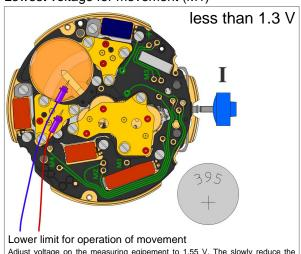
Adjust voltage on the measuring eqipement to 1.55 V. The slowly reduce the tension untill the movement stops
