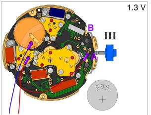
During connecton of +Pol to point A, the actual counter is turning, Short contact with +pole to point A Reduced the supply voltage to 1.3V to check the proper function of the counter. If the power supply is disconnected, the control mode must be starded again section 1.
