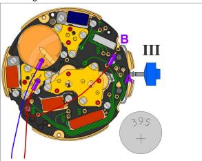
Change of active counter: M2-M3-M4-M2-M3- .After a timout of approx. 30 seconds since last contact, the control mode will be terminated.
