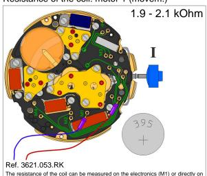
The resistance of the coil can be measured on the electronics (M1) or directly on the coils (electronic module must be removed).
